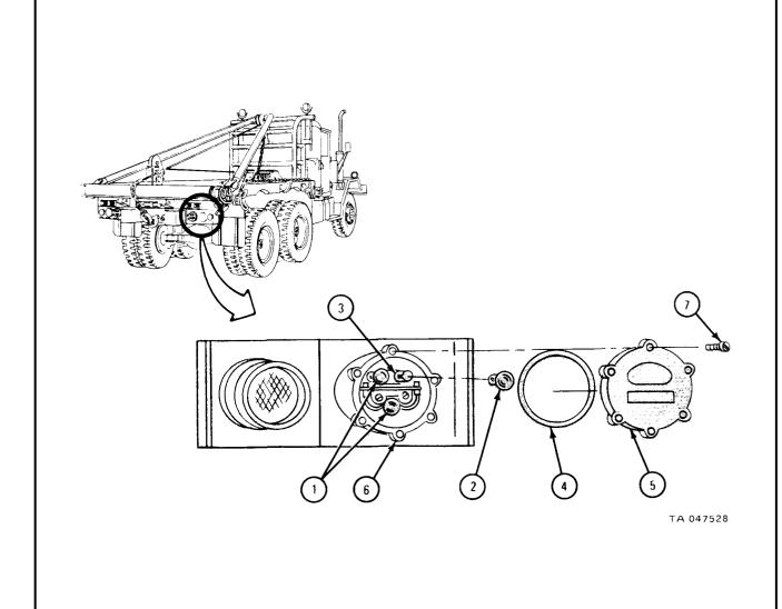
7-28. TAILLIGHT AND STOPLIGHT ASSEMBLY (LEFT SIDE ONLY) REMOVAL AND REPLACEMENT.
