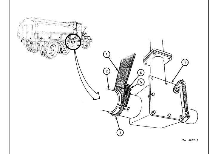
1. Using 9/16-inch wrenches, tighten three capscrews (1) with locknuts (2). GO TO FRAME 6
