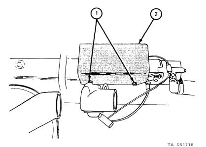
1. Using 1/2-inch wrench, loosen three capscrews (1) until intake manifold heater elbow (2) can be taken off mounting studs.
