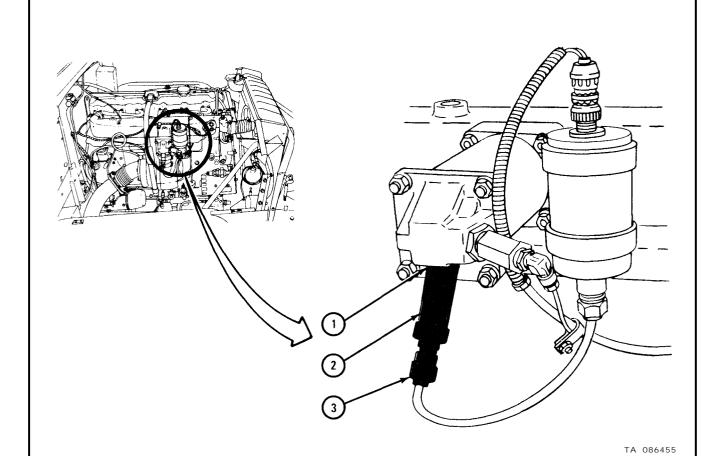
$^{4-15}$ . MANIFOLD HEATER (SIDE-MOUNTED) FUEL FILTER REMOVAL AND REPLACEMENT.
