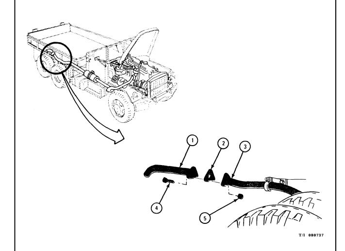
5-4. EXHAUST SYSTEM (HORIZONTAL) REMOVAL AND REPLACEMENT (TRUCKS M50A1, M50A2, AND M50A3).
