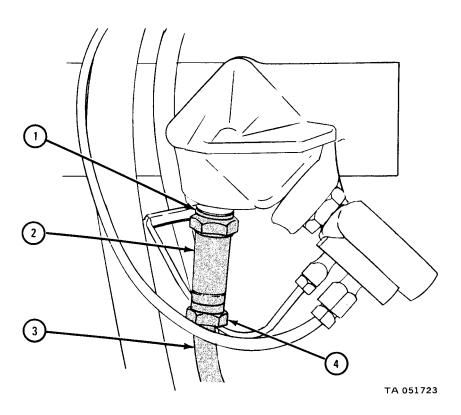
1. Using 1/2-inch wrench, tighten three capscrews (1).
