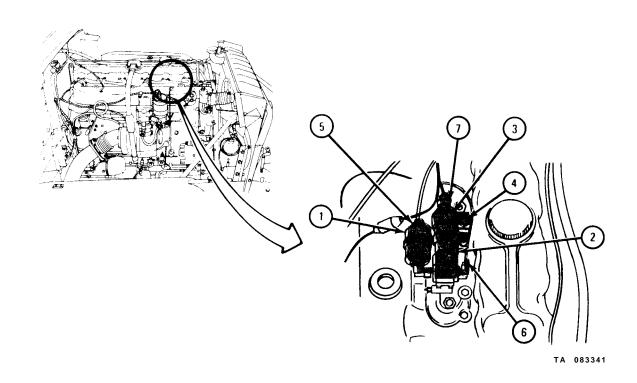
4-20. ENGINE MANIFOLD HEATER PUMP LINES AND FITTINGS REMOVAL AND REPLACEMENT (TRUCKS WITH ENGINES LDS 427-2 AND LDS 465-1).
