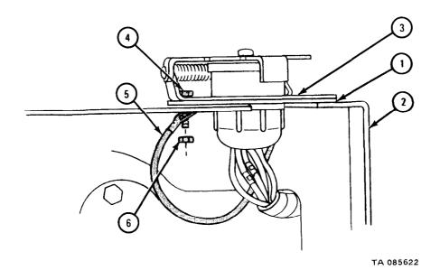
1. Put protector cover (1) in place and aline holes. Using 7/16-inch wrenches, screw in and tighten two screws (2) and two nuts (3).
