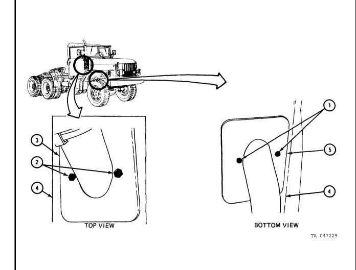
1. Using 1/2-inch wrench, unscrew two locknuts (1) and take off U-bolt and bracket (2).
