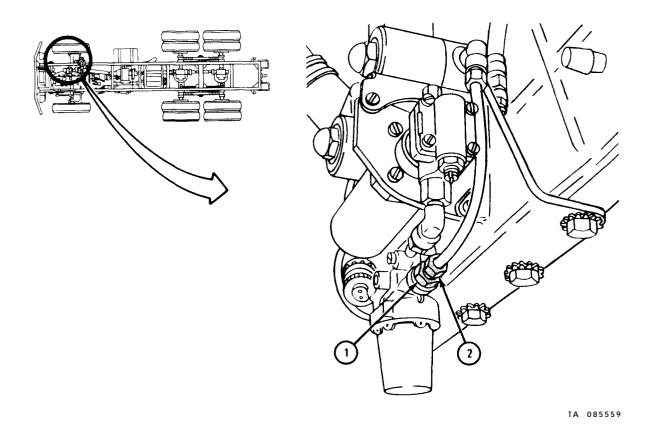
1. Working under truck using 9/16-inch wrench, screw on and tighten tube nut on fuel line (1).
