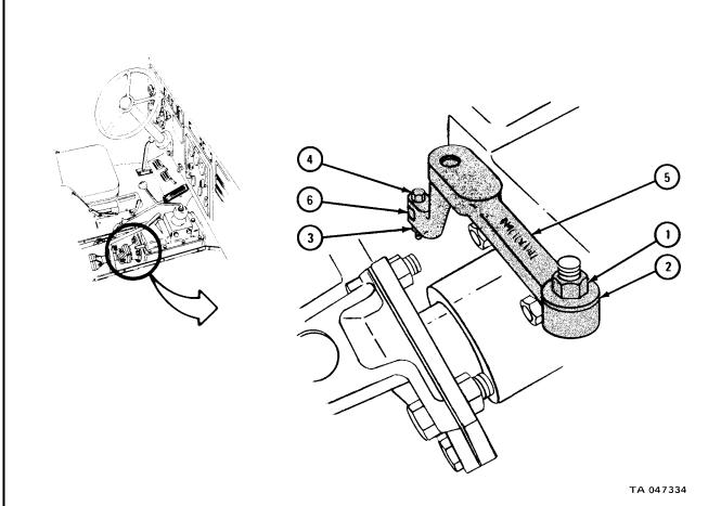
1. Using 3/4-inch wrenches, unscrew and take off locknut (1). Take out bolt (2) and take shift rod lever (3) away from linkage assembly (4).
