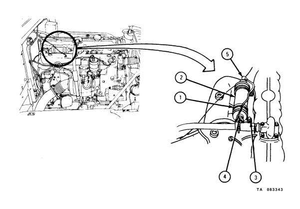
4-14. MANIFOLD HEATER (TOP-MOUNTED, UNCOVERED) SPARK PLUG REMOVAL AND REPLACEMENT (TRUCKS WITH ENGINES LDS 427-2 AND LDS 465-1).
