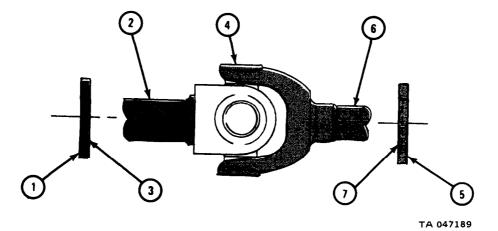
1. Using brass punch and hammer, put seal assembly (1) into end of axle housing (2) as shown.
