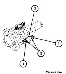
1. Place one side of yoke (1) on block of wood as shown.
