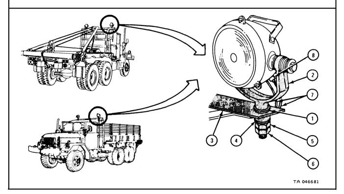
7-38. FLOODLIGHT HOUSING REMOVAL, REPAIR, AND REPLACEMENT (TRUCK M756A2).
