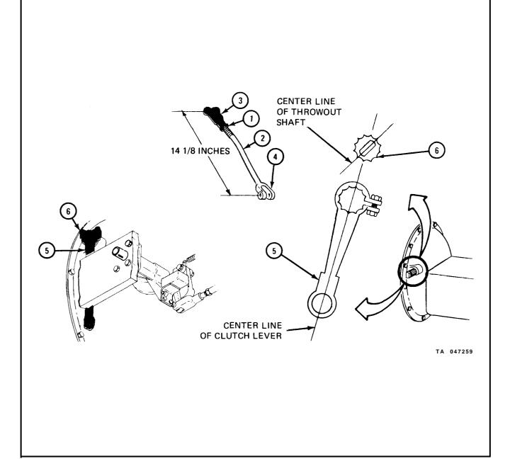
1. Push lower end of clutch throwout shaft lever (1) forward until resistance is noted. Using scale, measure distance from center of lever bottom hole to transmission flange as shown.
