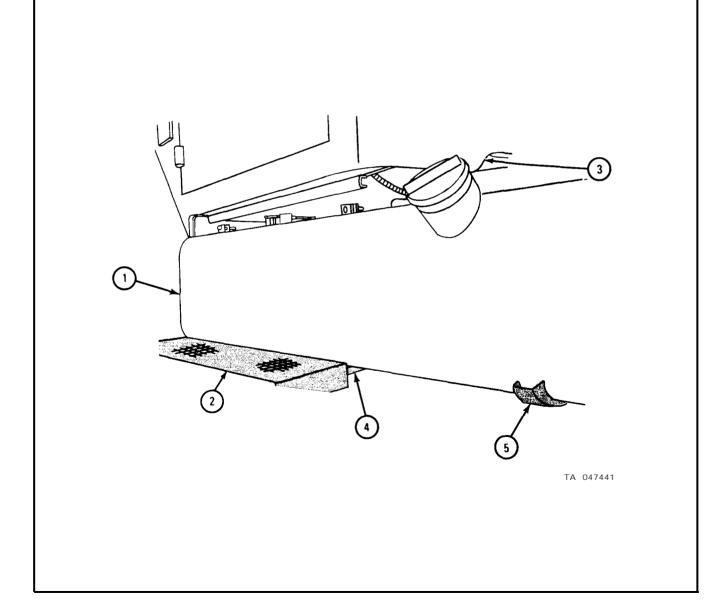
Soldier A 1. Using pry bar (1) between cab left rear sill (2) and frame rail (3), raise left rear of cab (4).
