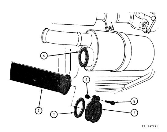
1. Join exhaust flex line (1) to elbow (2) using gasket (3) and coupling (4) as shown.
