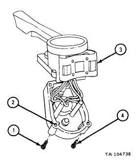
1. Check that contact points are not pitted or burned. If points are damaged, throw assembly away.
