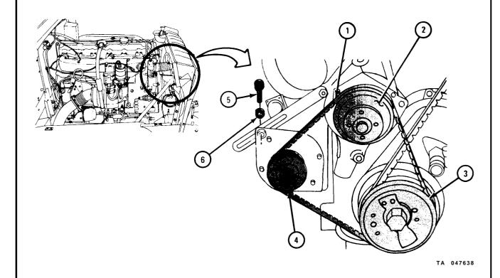
Place end of 30-inch bar (l) between crankcase (2) and generator (3). GO TO FRAME 3 TA 047639
