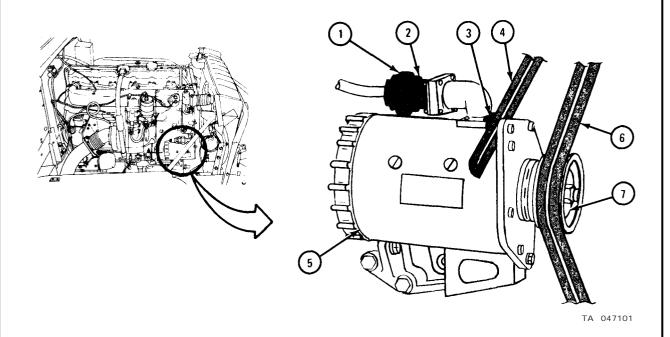
1. Using 5/8-inch socket wrenches, unscrew two nuts and washers (1) from bolts (2).
