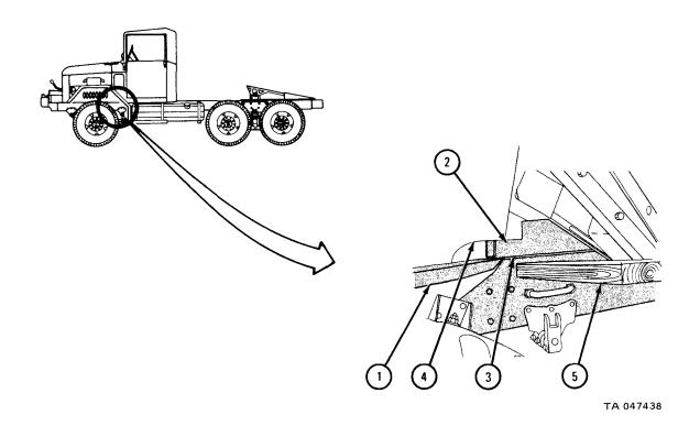
1. Using 15/16-inch wrenches and 6-inch ruler, hold two cab rear mounting screws (1) and tighten two nuts (2) until springs (3) are compressed to 1 25/32 inches.
