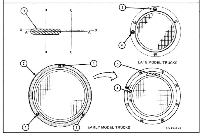
7-20. FRONT SERVICE SEALED BEAM REMOVAL AND REPLACEMENT.
