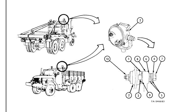
7-39. FLOODLIGHT SEALED BEAM REMOVAL, REPAIR, AND REPLACEMENT.
