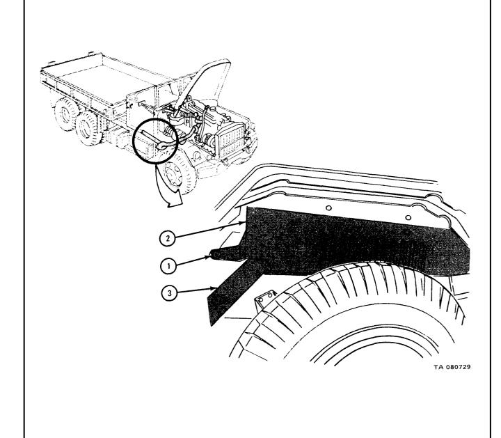
Soldier A 1. Using 9/16-inch wrenches, unscrew and take off three locknuts (1) and capscrews (2).
