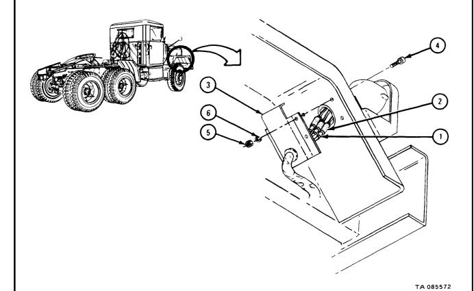
7-41. FRONT COMPOSITE LAMPS REMOVAL AND REPLACEMENT.
