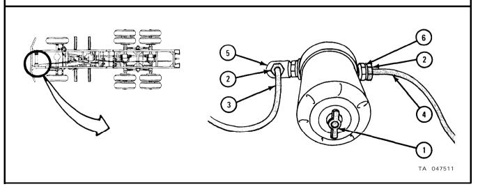
1. Using 9/16-inch wrench, unscrew and take off four screws and lockwashers (1). Take off primary fuel filter assembly (2).
