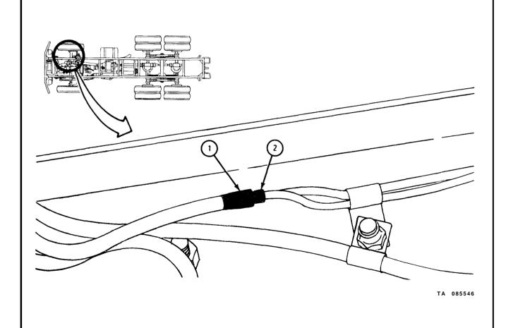
1. Working under truck and using 9/16-inch wrench, unscrew and take off fuel line (1) .
