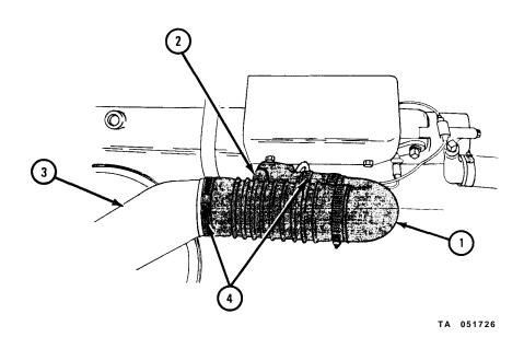
4-26. MANIFOLD FLAME HEATER (TOP-MOUNTED, COVERED) FUEL PUMP AND IGNITION UNIT REMOVAL AND REPLACEMENT (TRUCKS WITH ENGINES LD 465-1, LD 465-1C, AND LDT 465-1C).
