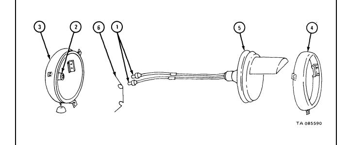
7-25. TAILLIGHT AND STOPLIGHT ASSEMBLY (RIGHT SIDE ONLY) REMOVAL AND REPLACEMENT (EARLY MODEL TRUCKS WITH TURN SIGNALS).
