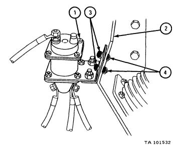
7-8. STARTER SWITCH REMOVAL, REPLACEMENT AND ADJUSTMENT (TRUCKS WITH PEDAL STARTER).
