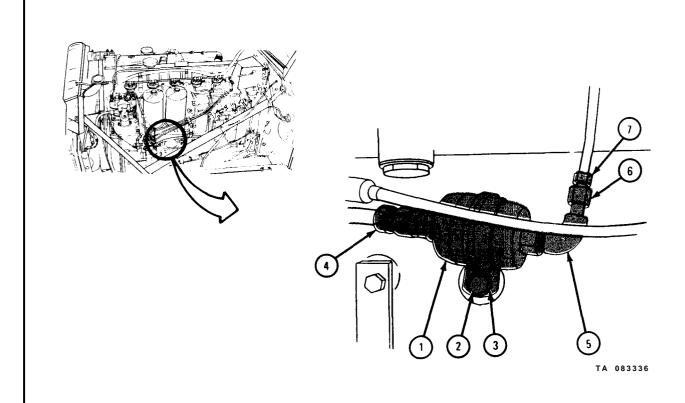
4-25. INTAKE MANIFOLD (TOP-MOUNTED, COVERED) FLAME HEATER AND ELBOW REMOVAL AND REPLACEMENT (TRUCKS WITH ENGINES LD465-1, LD465-1C, AND LDT 465-1C).
