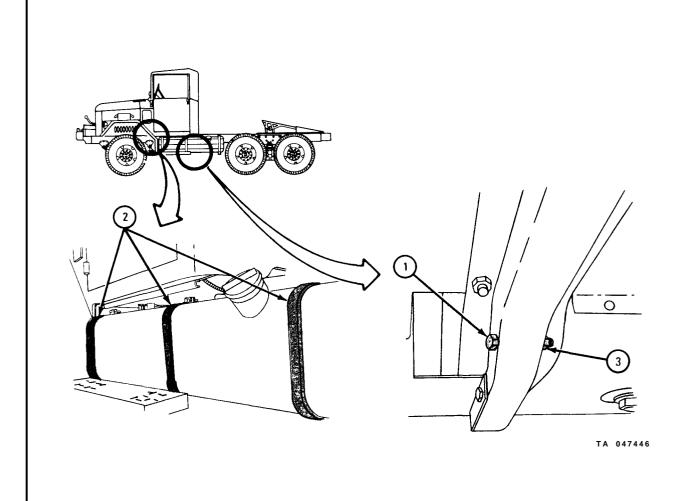
4-8. FUEL PUMP (IN-TANK) REMOVAL AND REPLACEMENT.
