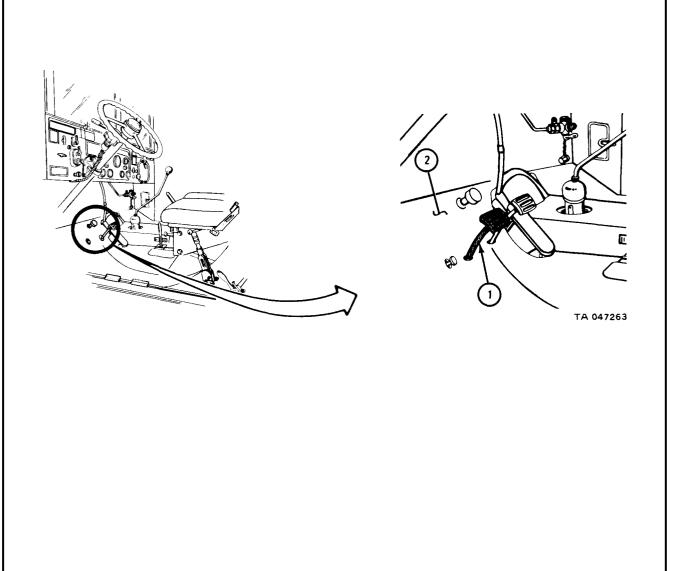
1. From underneath truck, put rubber bumper (1) on pedal shaft (2).
