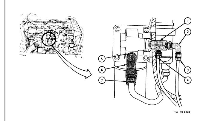
4-17. ENGINE MANIFOLD HEATER REMOVAL AND REPLACEMENT (TRUCKS WITH ENGINES LDS 427-2 AND LDS 465-1).
