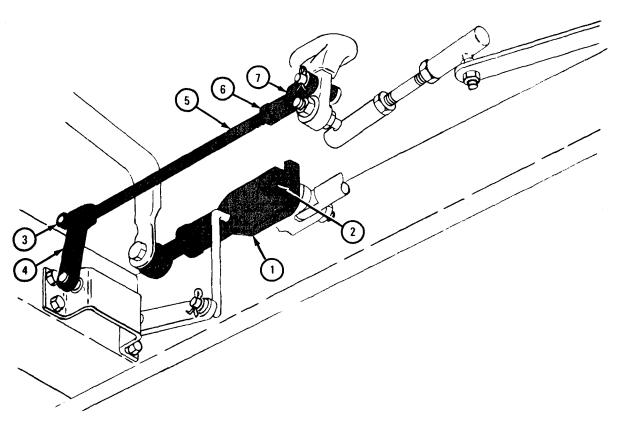
1. Using 3/4-inch wrenches, loosen two jamnuts (1).
