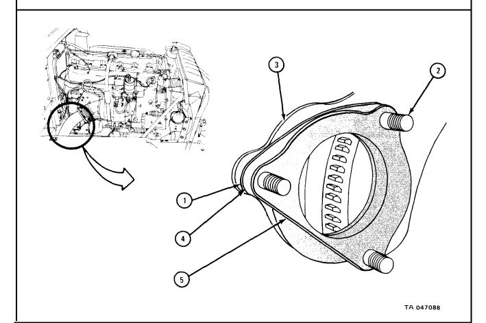
1. Put starter (1) in position. Aline three holes in starter mounting flange (2) with mounting studs (3). Lever (4) must be at top as shown.
