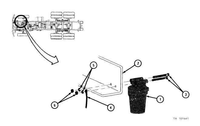
1. Working under truck using 9/16-inch wrench, hold adapter fitting (1). Using 7/16-inch combination box and open end box wrench, screw in and tighten tube nut (2).
