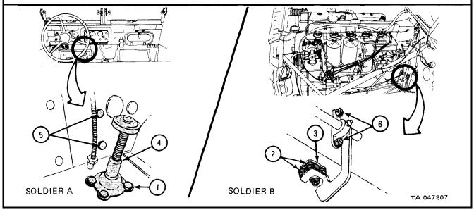
Soldier A 1. Using 7/16-inch wrench, hold two bolts (1) while soldier B unscrews locknuts (2).
