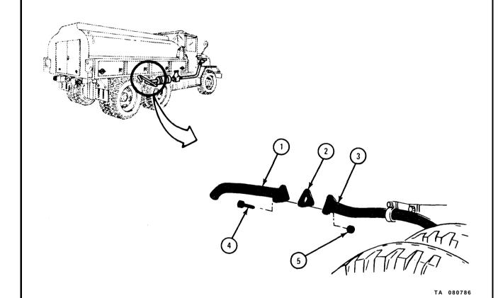
5-5. EXHAUST SYSTEM (HORIZONTAL) REMOVAL AND REPLACEMENT (TRUCKS WITH ENGINE LD 427).
