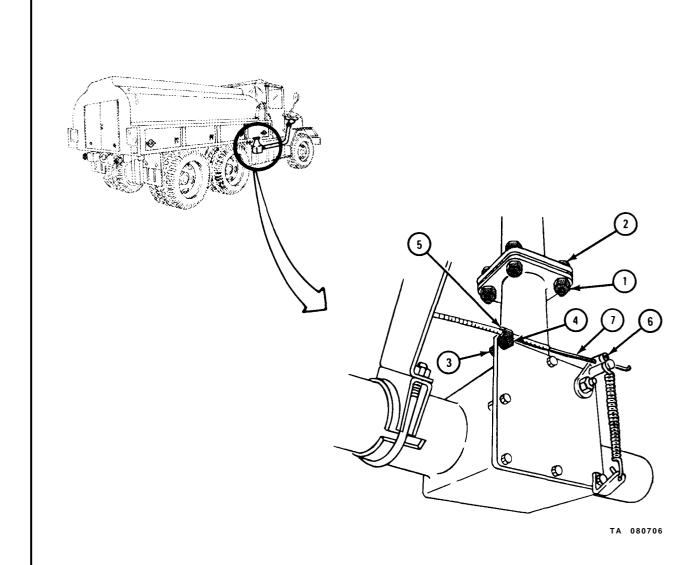
1. Using 9/16-inch wrench, unscrew and take off two nuts (1) and washers (2). Take off U-bolt (3) and bracket (4).
