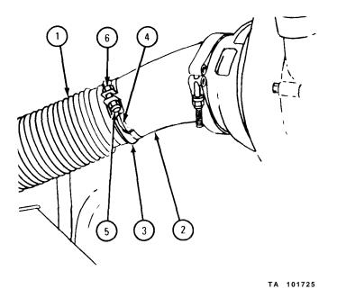
1. Turn elbow assembly (1) until exhaust flex line (2) is alined with exhaust pipe (3) and end of elbow assembly.
