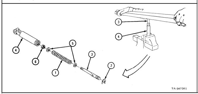
e. Assembly of Transmission Transfer Reverse Shift Rod (Transmission Transfers Without Air Actuated Positive Lockup).
