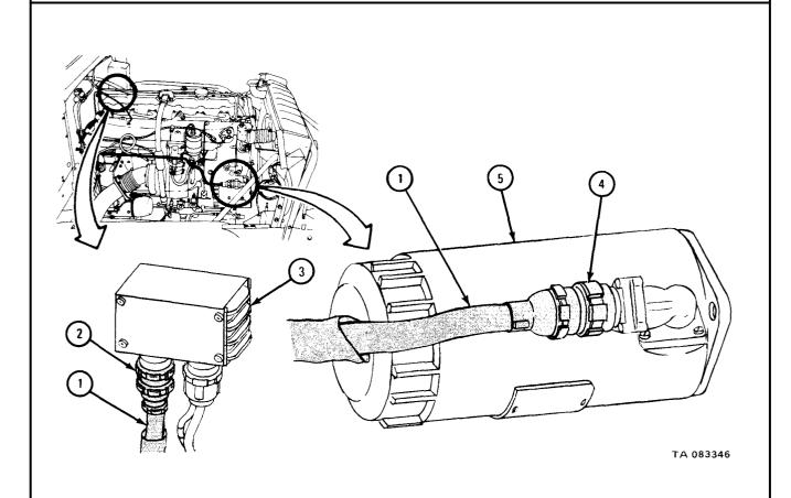
7-60. TRAILER CONNECTOR ELECTRICAL CABLE REMOVAL AND REPLACEMENT.
