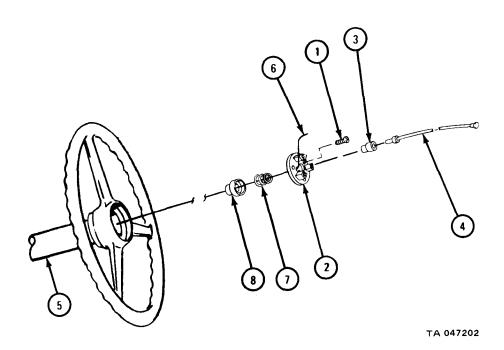
C. <u>Repair.</u> Repair the horn button by replacing any worn or damaged parts. The horn button parts kit contains all parts shown in this procedure except the cable. The cable must be ordered separately.
