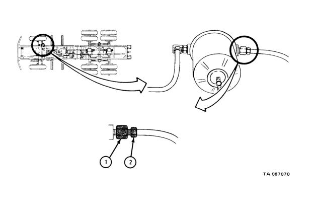
1. Using 7/8-inch open end wrench, hold tube coupling (1). Using 3/4-inch combination box and open end wrench, unscrew and take off tube nut (2).
