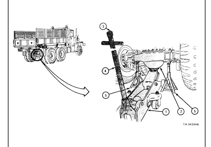
d. Removal of Rear Axle Housing Supports.
