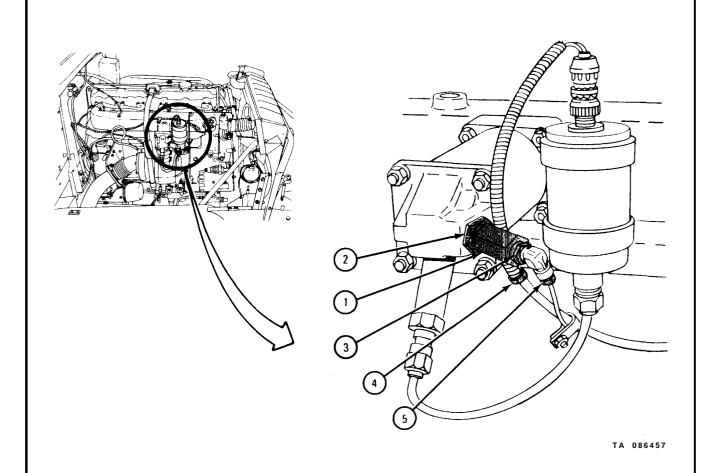
4-13. MANIFOLD HEATER (TOP-MOUNTED, UNCOVERED) IGNITION UNIT REMOVAL AND REPLACEMENT.
