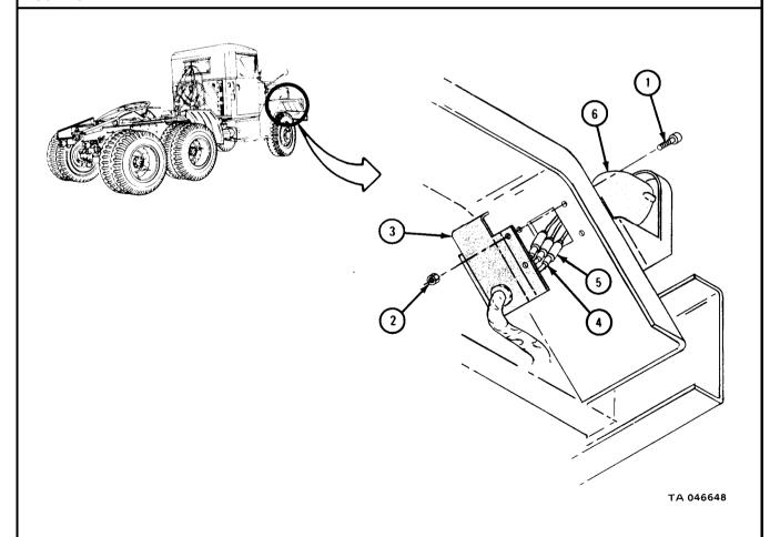
1. Using 9/16-inch wrench, unscrew and take off two capscrews (1) and lockwashers (2). Take light assembly (3) out of bracket (4).
