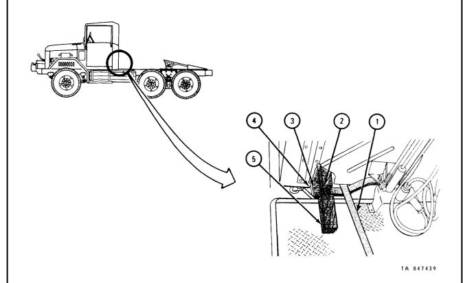
Soldier A 1. Using prybar (1) between cab left front sill (2) and frame rail (3), raise left front side of cab (4).
