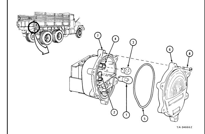
7-46. SERVICE AND BLACKOUT CLEARANCE LIGHTS REMOVAL AND REPLACEMENT (TRUCK M756A2).
