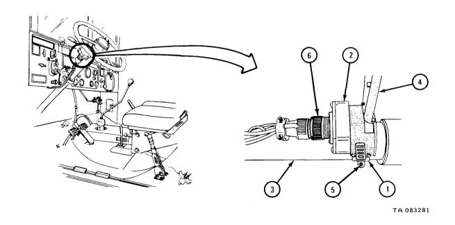
7-64. MANIFOLD HEATER SWITCH REMOVAL AND REPLACEMENT.
