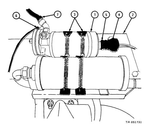
1. Put cover (1) in place. Using 1/2-inch wrench, screw in and tighten four capscrews and lockwashers (2) .
