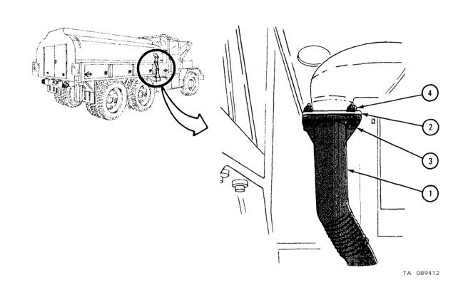
1. Using 3/4-inch wrenches, tighten four capscrews (1) with locknuts (2). GO TO FRAME 11
