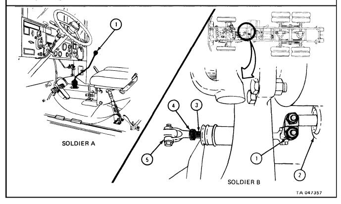
9-7. TRANSMISSION TRANSFER OUTPUT COVER SEAL AND AIR VENT REMOVAL AND REPLACEMENT.
