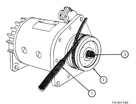
1. Hold generator (1) by hand and set it on mounting bracket (2).
