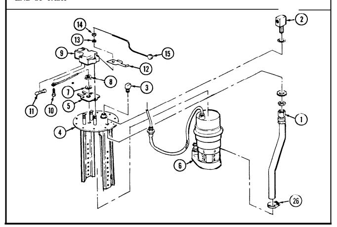
4-9. FUEL PUMP (IN-TANK) FUSE REMOVAL AND REPLACEMENT.
