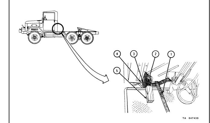
Soldier A 1. Lift rear end of fuel tank (1) and take it out of rear support bracket (2).
