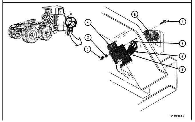
1. Using 9/16-inch wrench, unscrew and take out two capscrews (1) and lockwashers (2). Take light assembly (3) off bracket (4).
