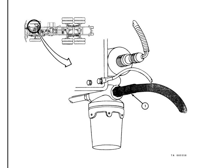
1. Working under truck using 9/16-inch wrench, hold nut (1). Using 7/16-inch combination box and open end box wrench, screw on and tighten tube nut (2).
