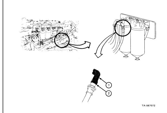
1. Using 3/4-inch open end wrench, hold hose nut (1). using 5/8 inch combination box and open end box wrench, screw on and tighten tube nut (2).
