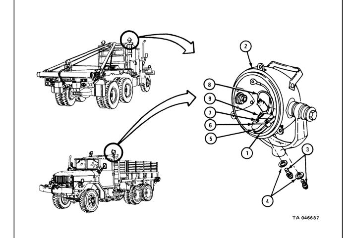
7-67. HYDRAULIC STOPLIGHT SWITCH REMOVAL AND REPLACEMENT (ALL TRUCKS EXCEPT MODELS M275A1 and M275A2).
