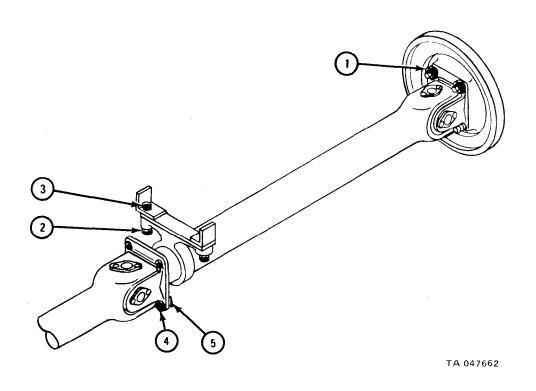
10-4. PROPELLER SHAFT AND UNIVERSAL JOINTS REMOVAL AND REPLACEMENT (ALL EXCEPT INTERMEDIATE PROPELLER SHAFT ON TRUCK M36A2).
