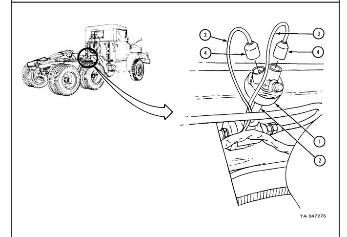
7-69. LOW AIR PRESSURE BUZZER SWITCH REMOVAL AND REPLACEMENT.
