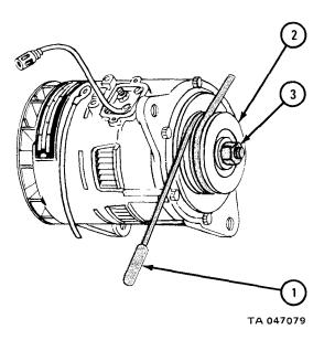
1. Hold alternator (1) by hand and set it on mounting bracket (2) in engine compartment as shown.
