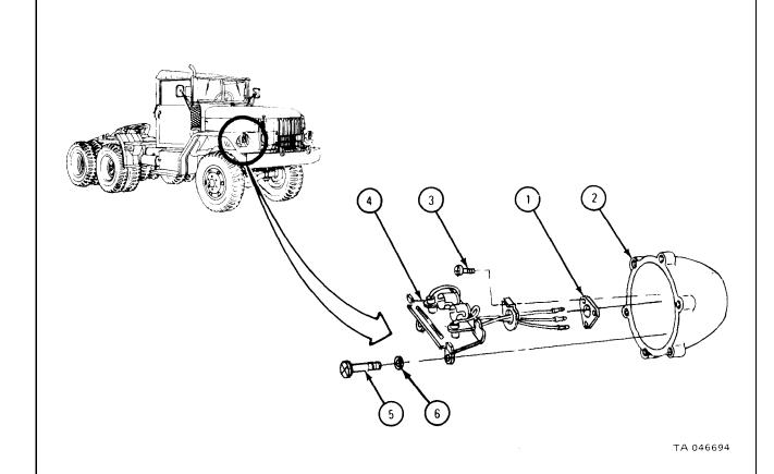
7-37. FLOODLIGHT AND BRACKET ASSEMBLY REMOVAL, REPAIR, AND REPLACEMENT (TRUCK M756A2).
