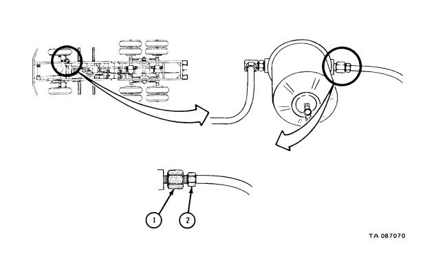
1. Using 7/8-inch open end wrench, hold coupling (1). Using 3/4-inch combination box and open end box wrench, screw on and tighten tube nut (2).
