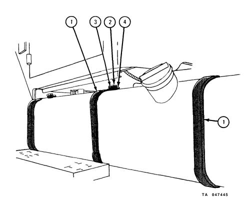
1. Using 1/2-inch wrenches, hold screws (1) on forward, center, and rear straps (2) and tighten nuts (3).
