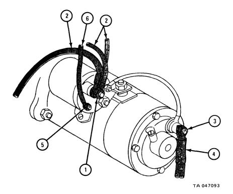
1. Using 15/16-inch socket wrench, unscrew and take off three nuts and lockwashers (1).
