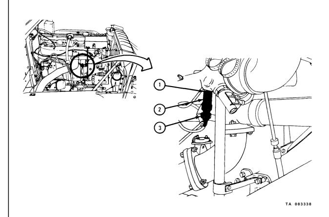
4-24. MANIFOLD HEATER (TOP-MOUNTED, COVERED) FUEL FILTER REMOVAL AND REPLACEMENT.
