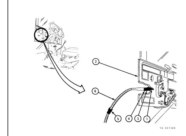
Soldier A 1. Put throttle control cable (1) through hole in floor and slide floor fitting (2) down throttle control cable into hole.
