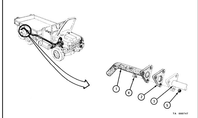
5-6. EXHAUST SYSTEM (VERTICAL STACK) REMOVAL AND REPLACEMENT (TRUCKS WITH ENGINES LD 465-1, LD 465-1C, AND LDT 465-1C EXCEPT TRUCKS M50A2 AND M50A3).
