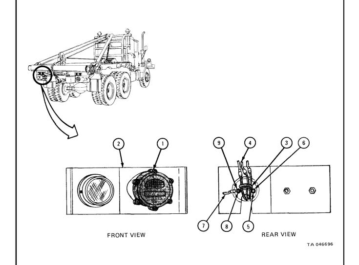
7-29. TAILLIGHT AND STOPLIGHT LAMP (LEFT SIDE ONLY) REMOVAL AND REPLACEMENT.
