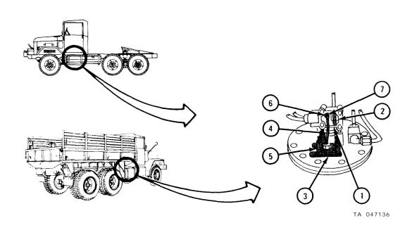
1. Put cover (l) over four studs (2) and seat cover firmly on gasket (3).
