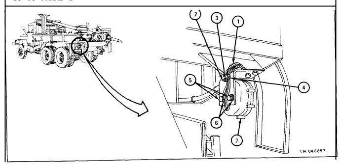
1. Using 9/16-inch wrenches, hold two nuts (1) and unscrew and take off two capscrews (2). Take off bracket (3).
