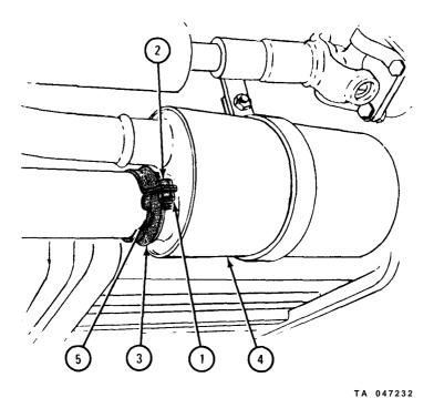
1. Using 9/16-inch wrenches, unscrew and take off two locknuts (1) from two bolts (2).
