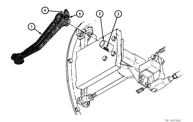
1. Put pedal (1) through hole in cab floor (2).
