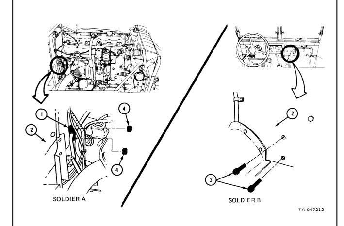
7-7. MAGNETIC STARTER SWITCH REMOVAL AND REPLACEMENT.
