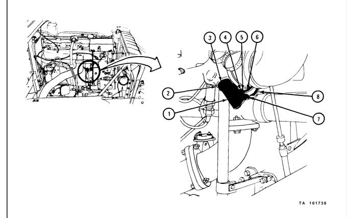
4-22. MANIFOLD HEATER IGNITION UNIT REMOVAL AND REPLACEMENT (TRUCKS WITH ENGINES LDS 427-2 AND LDS 465-1).
