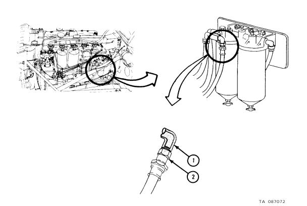
1. Using 11/16-inch open end wrench, hold hose nut (1). Using 3/4-inch combination box and open end box wrench, unscrew tube nut (2) and take off fuel hose (3).
