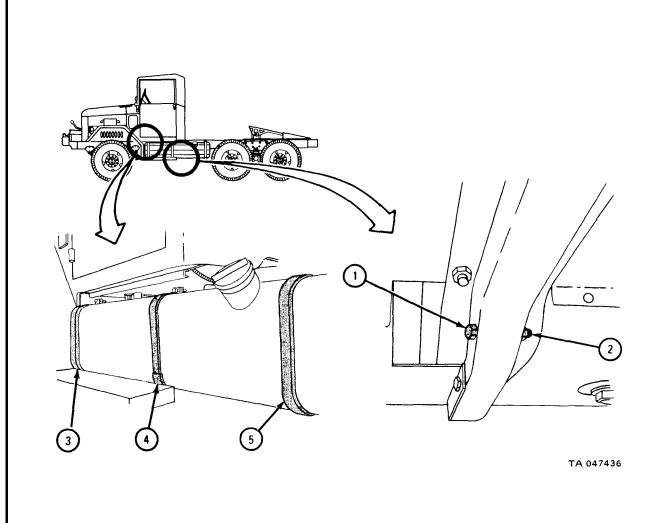
1. Working under cab rear crossmember (1) using 15/16-inch wrenches, loosen two nuts (2) as much as possible without taking them out.
