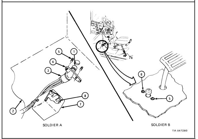
7-66. FLOODLIGHT HOUSING SWITCH REMOVAL, REPAIR, AND REPLACEMENT (TRUCKS M756A2 AND M764).
