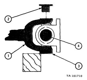
1. Place one side of yoke (1) on wood block as shown.
