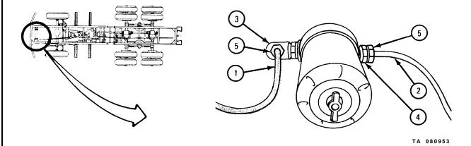
e. Replacement of Secondary and Final Fuel Filter Assemblies.
