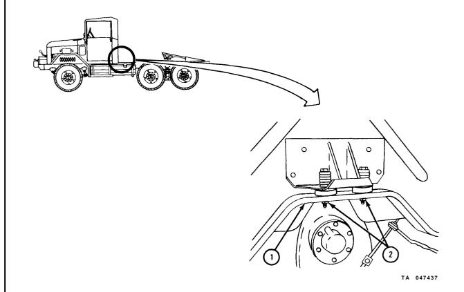
Soldier A 1. Using prybar (1) between cab left front sill (2) and frame rail (3), raise left side of cab (4) about 3/4 inch.
