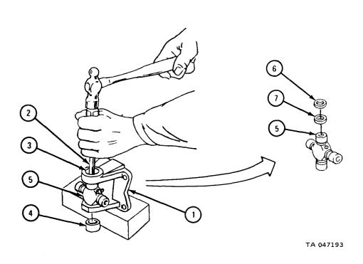
b. Disassembly (Bearing Cap Type).
