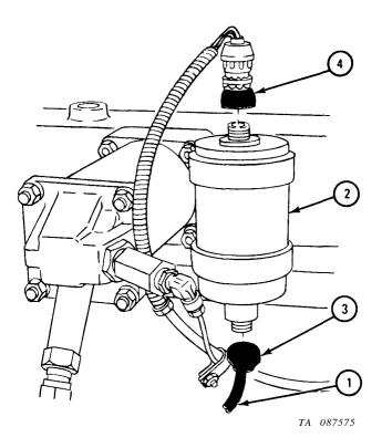
4-23. MANIFOLD HEATER (TOP-MOUNTED, COVERED) SPARK PLUG REMOVAL AND REPLACEMENT.
