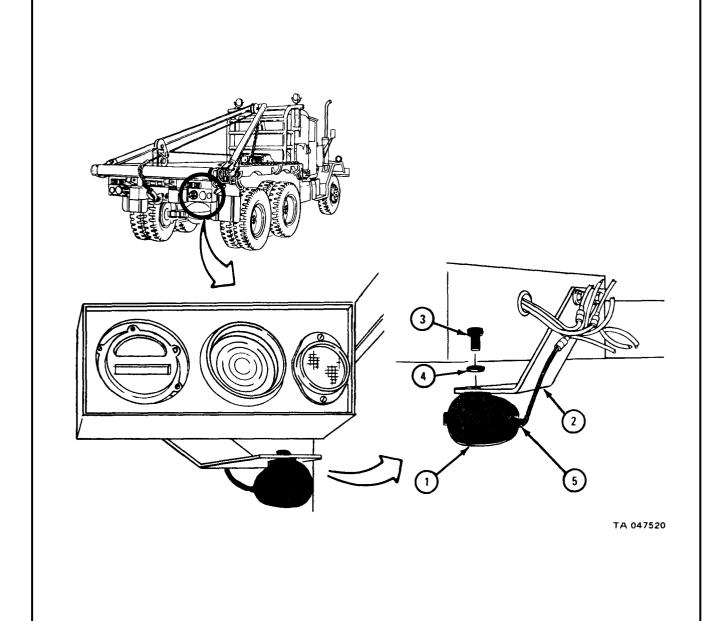
7-32. BLACKOUT STOPLIGHT LAMP (RIGHT SIDE ONLY) REMOVAL AND REPLACE-MENT (EARLY MODEL TRUCK WITH TURN SIGNALS).
