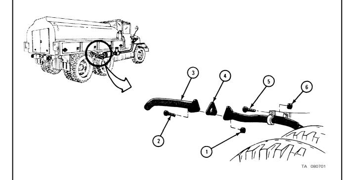
1. Working under truck and using 1/2-inch wrench, unscrew and take off two nuts (1), two washers (2), and clamp bracket (3). Take off U-bolt (4).
