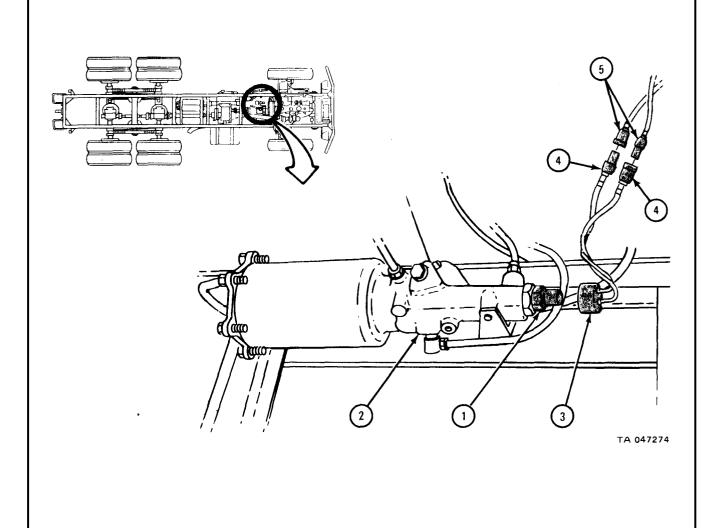
7-68. AIR STOPLIGHT SWITCH REMOVAL AND REPLACEMENT (TRUCKS M275A1 AND M275A2).
