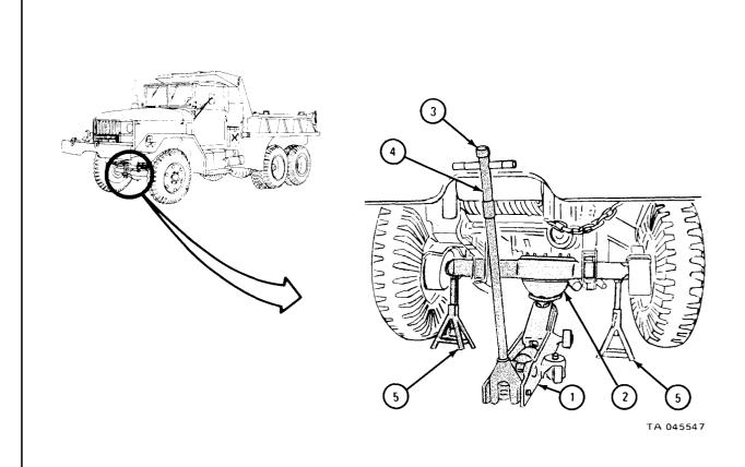
c. Jacking and Supporting Rear Axle Housing.
