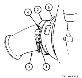
1. Using 9/16-inch wrench, unscrew and take off two locknuts and flat washers (1).
