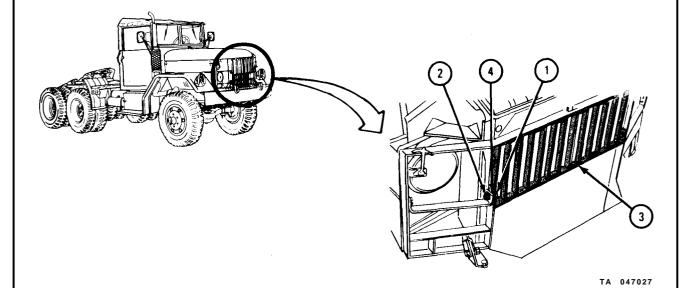
1. Using 3/4-inch box wrenches, loosen two nuts (1) on two bolts (2) at left and right side of brush guard (3).
