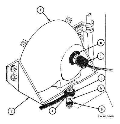
7-22. BLACKOUT DRIVE LIGHT ASSEMBLY AND BRACKET REMOVAL AND REPLACEMENT (TRUCKS WITHOUT WINCH).
